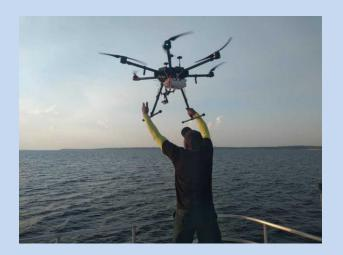
Figure 2. The AQB (the white box) was carried on a multirotor UAV to monitor the vertical distribution on the Amazon River (Zhao et al. 2021)
